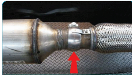
Check the mid-joint connection for an exhaust leak
