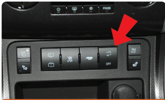
The power liftgate disable switch in the Off position.
