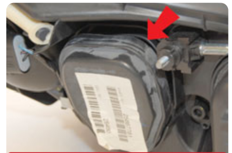
Low beam cover loose
