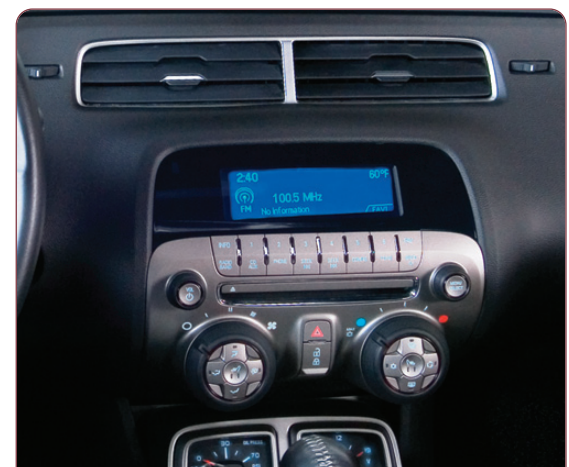
Do not point the center vents down to help avoid radio display fogging.
