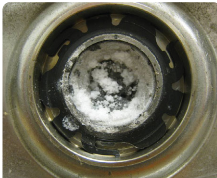
Crystalline urea deposits over the DEF injector's exit nozzle
