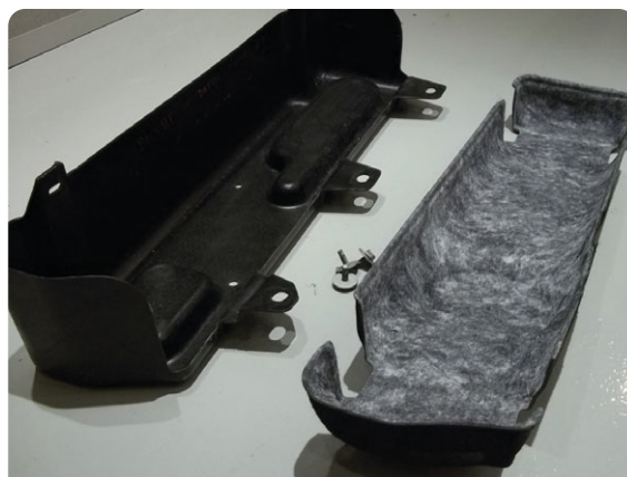
DEF tank shield and insulator
